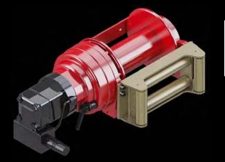
This range of pulling winches has a line pull capacity of between 1 and 30 . The design incorporates three independent components (hydraulic motor, static brake and planetary gearbox) to provide maximum reliability and easy maintenance.
