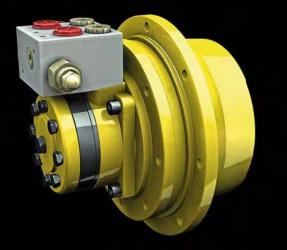
Wheel drives come in 5 sizes with a maximum torque ranging between 800 and 3,500 Nm. These models are suitable for track drive and wheel drive applications due to the relatively high load supported by the bearings (8,000 kg in the EH models). Several accessories are available (including static brake, disengagement system, and control valves).
